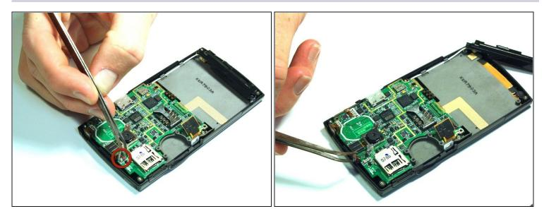
• Use the <u>tweezers</u> to unsnap the connection between the motherboard and the speaker. The speaker is attached to the front casing.
