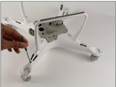
• Remove the eight 7 mm hex screws by turning counterclockwise with a 2 mm hex bit.
