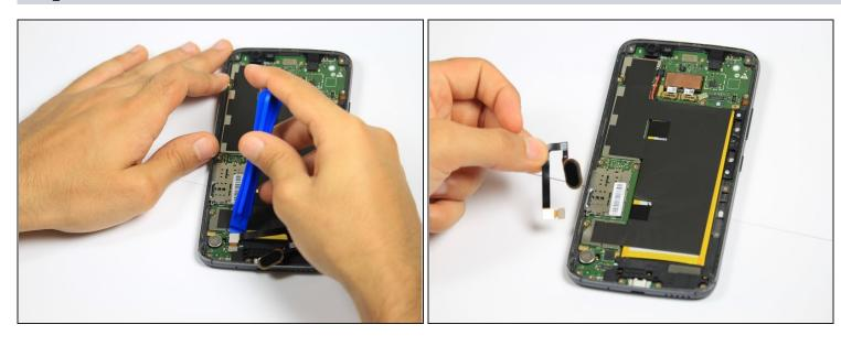
• Remove the fingerprint connector by gently prying underneath the connector with the opening tool.
