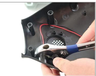
Using an adjustable wrench, remove the nut on the back of the power button by rotating the nut counterclockwise.
