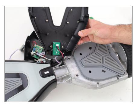
Lift both the left and right sides of the top half of the shell from the hoverboard's chassis.
