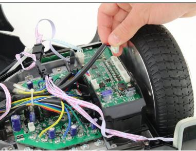
Remove the red and black sleeved connector from the sensor assembly by squeezing the tab and pulling up.
