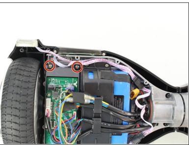
Remove the four 7mm screws by using a Phillips #2 screwdriver to rotate the screws counterclockwise.
