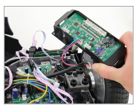
Remove the sensor assembly on the motherboard side of the hoverboard by gently lifting and pulling away from the hoverboard. To reassemble your device, follow these instructions in reverse order.
