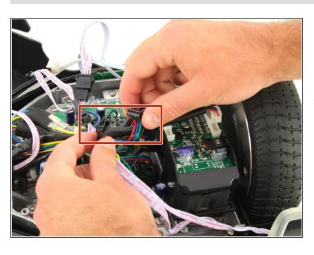
Remove the red, blue, and green cable from the extension connected to the sensor assembly by
