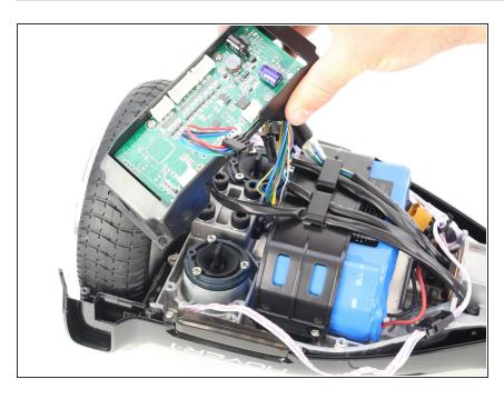
Remove the sensor assembly on the battery side of the hoverboard by gently lifting and pulling away from the hoverboard.
