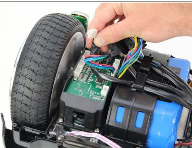
On the battery side of the hoverboard, remove the red, black, and purple sleeved cable from the sensor assembly by squeezing the tab and pulling up.
