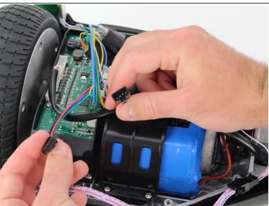
Remove the red, blue, and green cable from the cable extension connected to the sensor assembly by squeezing the tabs on the side of the connector.
