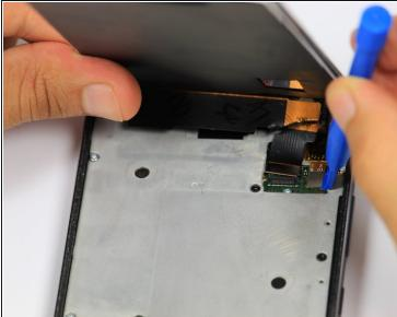
Disengage the two cable connectors by gently prying beneath the edge of the connector with the opening tool.
