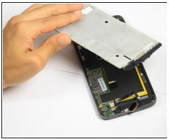
• Grab ahold of the fingerprint sensor and push it through the opening in the metal cover.
