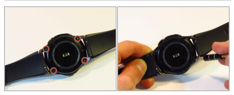
Remove the four 4.2mm screws with a Y00 screwdriver.
