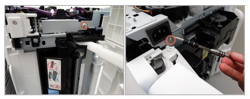
Remove two Phillips #2 10mm from the left (front) and right (back) side that attach the power module to the printer.
