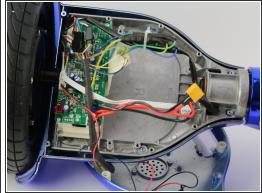
Remove the battery out of the hoverboard by lifting the battery then sliding it out from under the wires.
