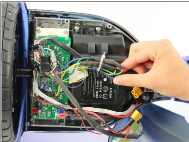
Remove the bundle of wires from the clip on the top of the battery.
