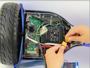
Unplug the battery from the gyroscope/motherboard by holding the yellow connector and pulling apart.
