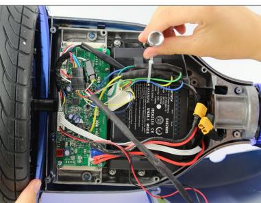
Using a Phillips #1 screwdriver, remove the four 14 mm screws that hold the battery on the device.
