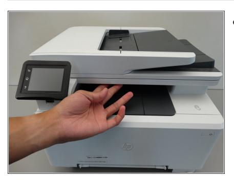
Lift up the top of the printer by pulling up on it.
