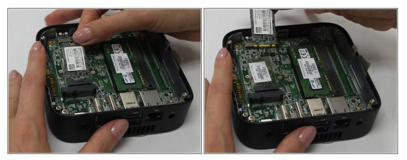
• Pull the hard drive at an angle to remove it from its slot.
