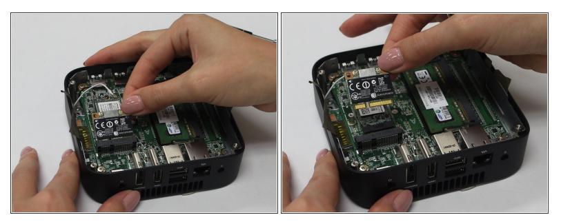
• Remove the WLAN module by pulling it away from the slot at an angle.
