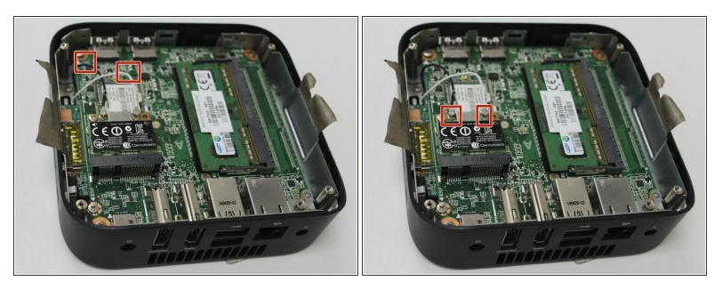
Disconnect the white and black antenna cables from the module.
