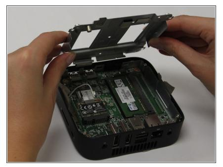
Insert your spudger into the gap between the bottom shield and the ports and gently pry to lift and remove the shield.
