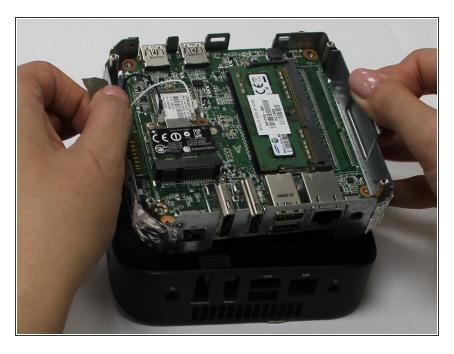
• Use the mylar tape to lift the system board out of the computer.
