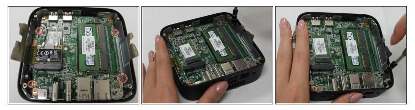
Remove the four Phillips M2.5×4.0 screws by using the Phillips #1 Screwdriver, that secure the system board to the computer.
