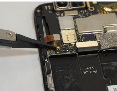
Using a set of tweezers, pull off the small piece of tape on top of the ribbon cable connector on the left side of the motherboard.
