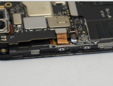
• Use a plastic opening tool or spudger to scrape the glue away from the ribbon cable.
