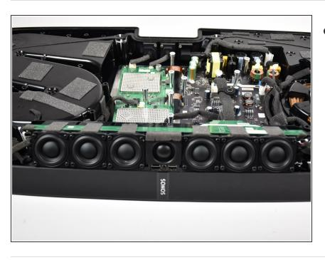
Prop the removed main speaker array up on top of the main circuit board.
