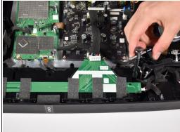
Remove the two 16mm T-20 screws located on both sides of the main speaker array by turning counter-clockwise.
