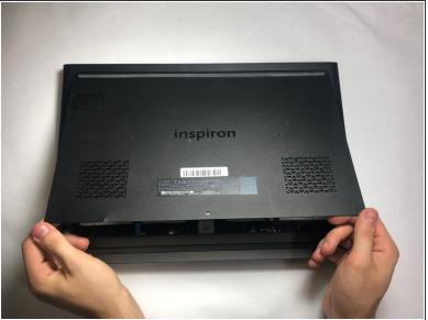
Remove the panel by lifting up the side towards you
