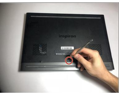
Remove the 3mm screw on the back using a Phillips #1 screwdriver.
