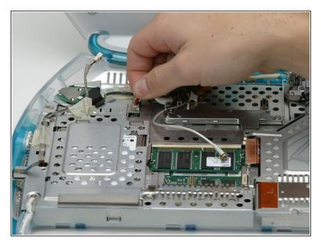
Disconnect the large display data cable from the logic board and deroute it from the plastic and metal tabs.
