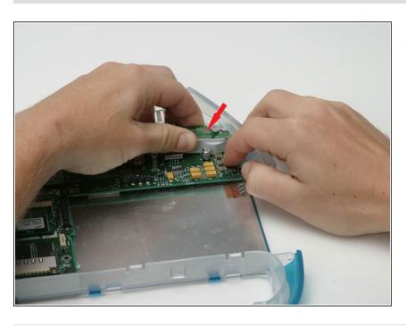
Push down firmly on the logic board and pull the DC-In board up from its connectors and then to the left.
