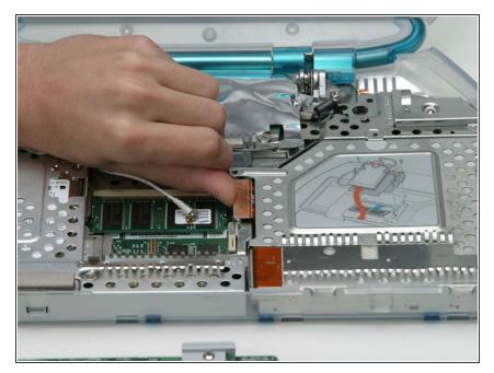
Disconnect the optical drive cable from the logic board.
