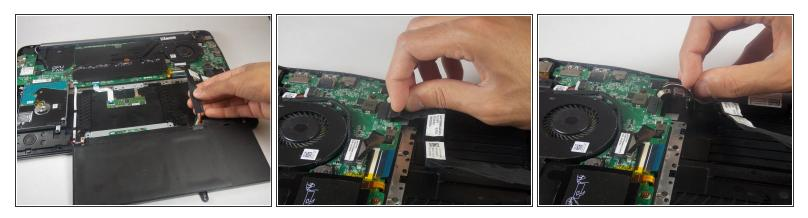
Pull the battery cable's pull tab towards the battery to disconnect it from the motherboard.
