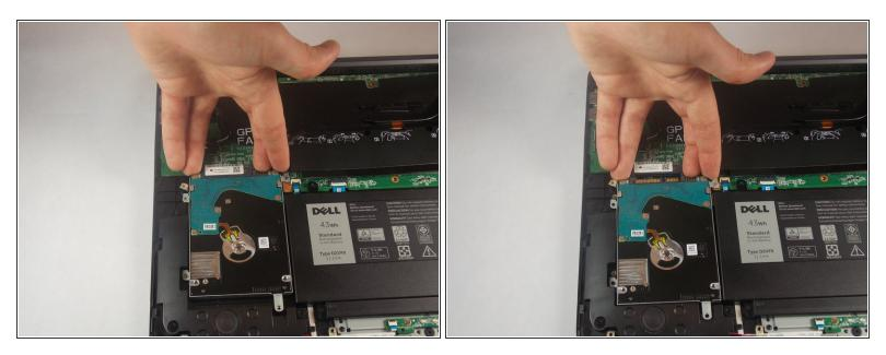
Disconnect the hard drive from the motherboard by placing your fingers at the back, and pulling forward towards the front of the chassis.
