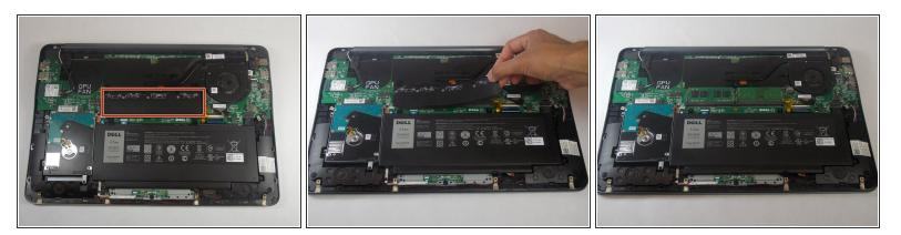
Remove the plastic heat spreader that covers the RAM sticks.
