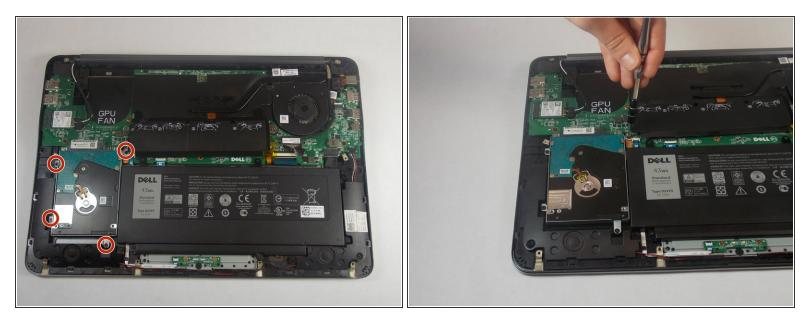
• Remove the four 5.0 mm-long Philips #0 screws connecting the hard drive to the chassis.
