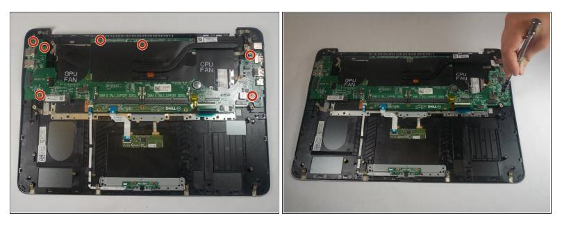
• Remove the seven 3.0 mm-long Philips #0 screws that secure the motherboard.
