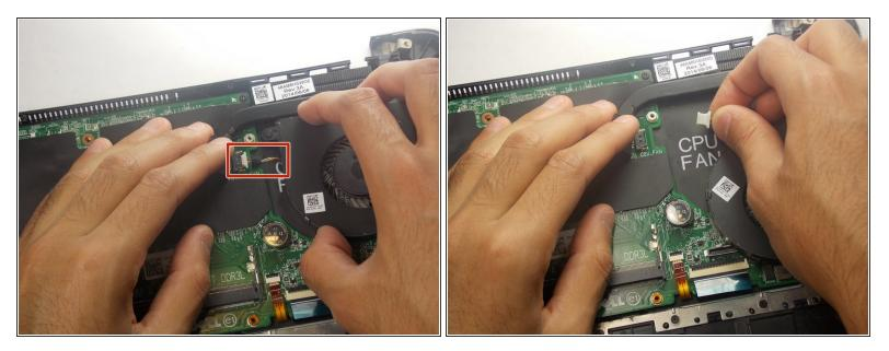
Disconnect the wire that connects the fan to the motherboard. This can be found under the flap directly to the left of the fan.
