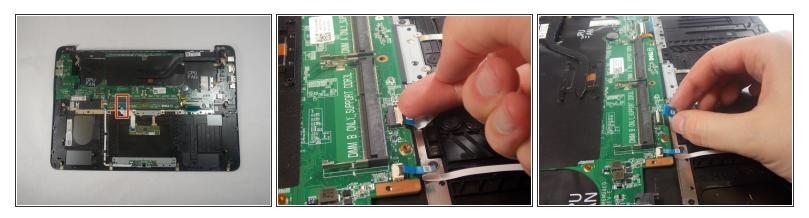
• Unlatch the ribbon cable by pulling the white release up.
