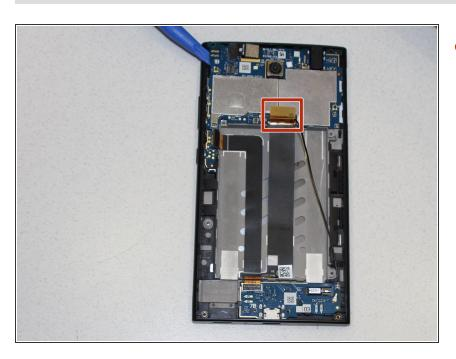
Unclip circuit connectors from phone to motherboard.
