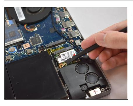
Disconnect the wires connecting the card to the motherboard.
