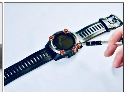
Use a T6 screwdriver to remove the five 1.7 mm screws from the watch face.
