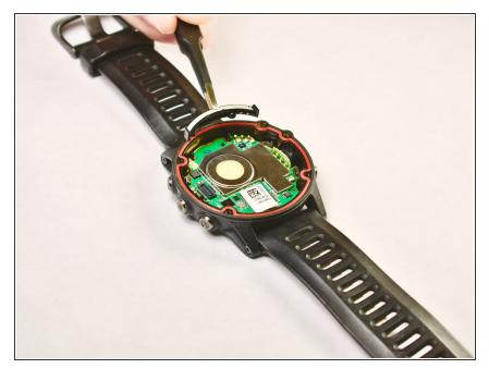
Locate the antenna, which is located on the motherboard.
