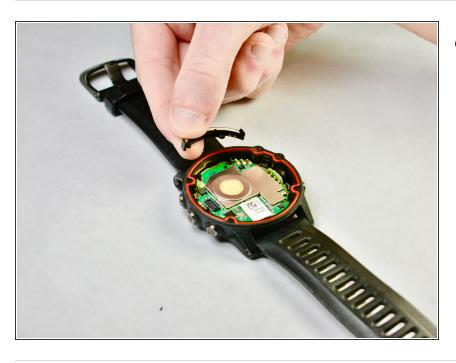
Carefully remove the antenna, and set it aside.
