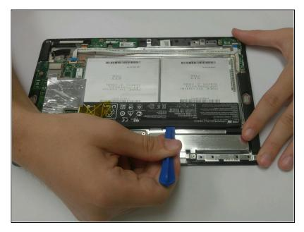
Insert the iFixit Opening Tool underneath the top of the battery and gently lift upwards to remove the battery.
