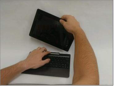
• Remove the tablet portion of the device from the keyboard by pushing the large silver button near the base of the tablet. Pull up on the tablet to remove from the keyboard.
