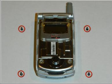
On the display housing, locate and unscrew the four corner T6 Torx screws connecting the housing and the internal cover.
