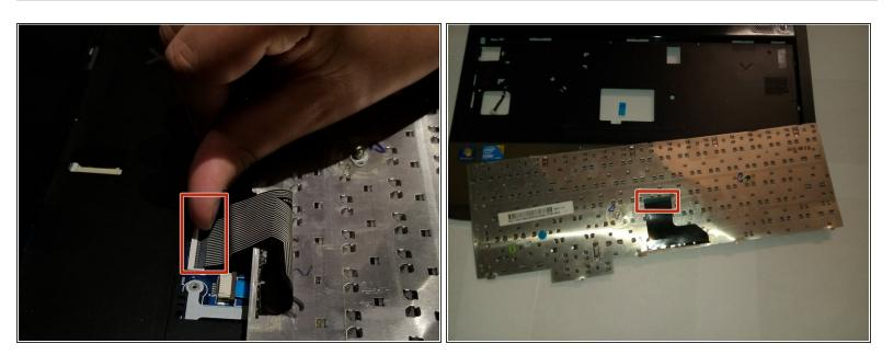
• Disconnect the keyboard cable from the motherboard.
