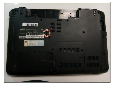
Remove securing screw with the PH0 head.
