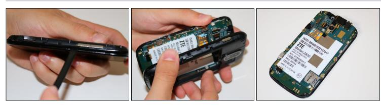
• Notice the crease in the shiny black plastic. Insert the flat end of your spudger here, about 3mm above the volume buttons, and work your spudger around the circumference of the phone until the front and back are separated.
