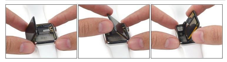
• Fold the screen up and over to the right, to expose the cables underneath.
