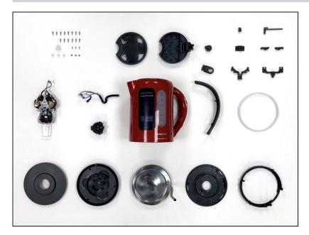
• The kettle is now fully disassembled.
