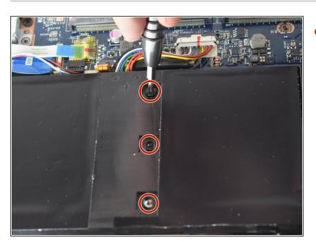
Remove the three 4 mm Phillips #1 screws securing the battery.
