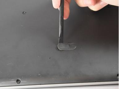
Remove the top and middle rubber feet under the laptop to reveal hidden screws.
