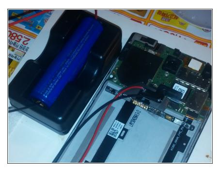
The built-in battery was tested with a meter (electric tester). The external battery is connected directly without going through the battery protection circuit, so the mobile phone boots normally.
