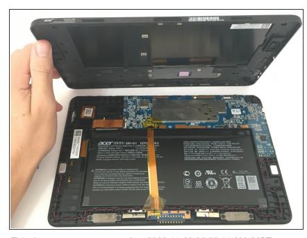
Set the device screen side down and remove the back casing.
