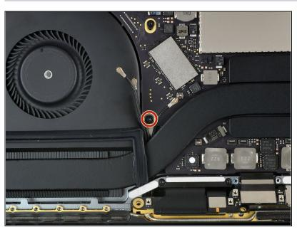
Remove the 2.8 mm T5 Torx screw securing the three antenna coax cables to the main board.
