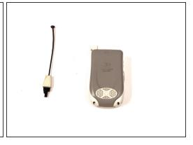
Remove the antenna by grasping from the white plastic piece just below the antenna and pulling away from the phone.
