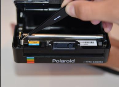
• Remove the left and right springs with a pair of tweezers.
