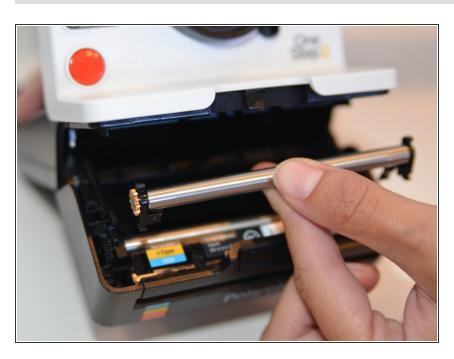
Lift out the top roller. The gold and black pieces will remain attached to the roller.
