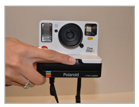
Pull the hinge button over to open the camera.
