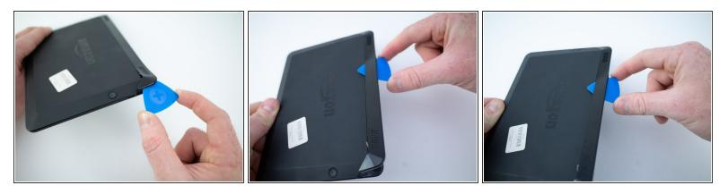
Insert an opening pick underneath the speaker bezel, and slide it along the perimeter to separate it from the tablet.
