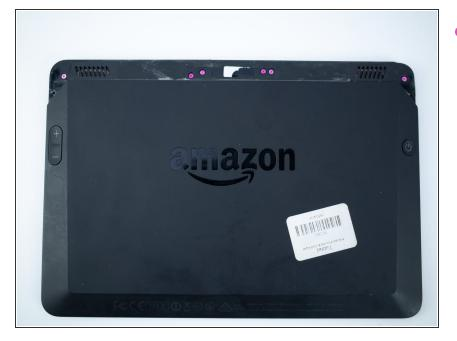
Remove the six pink 3mm T3 Torx screws from the back case.
