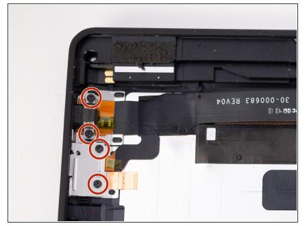
Remove the four 2.3mm T5 Torx screws from the micro USB port and power button assembly.
