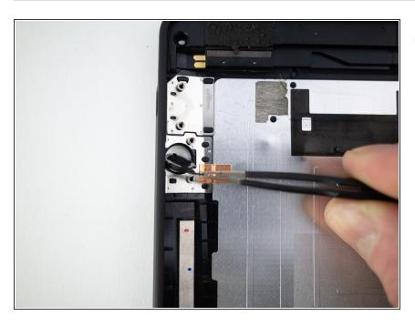
• Remove the power button from the rear panel.
