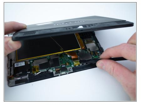
Use the flat end of a spudger to pry up and disconnect the rear panel press-fit connector from the motherboard.
