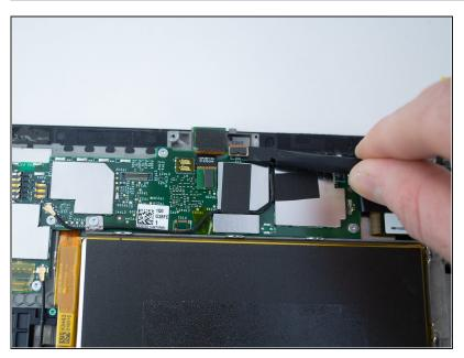
Pry up the ambient light sensor press-fit connector from the motherboard with the flat end of a spudger.
