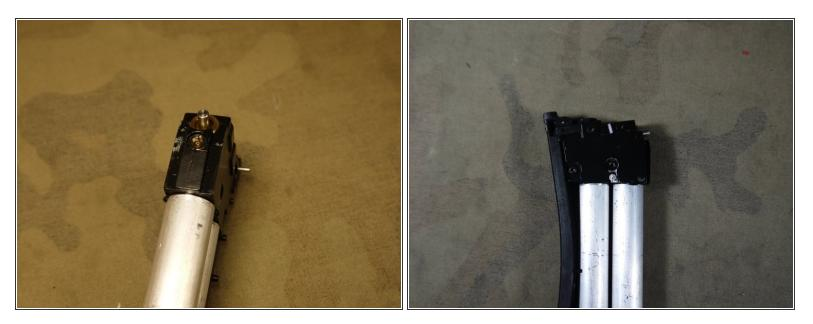
• Now add the plastic top section back onto the mag and add the pin to hold it in place.
