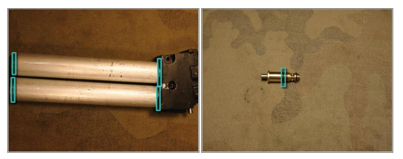
• If you are still struggling with leaks. You can use Teflon tape on the treads and silicone based plumbers grease on O-rings that do not move back and forth.
