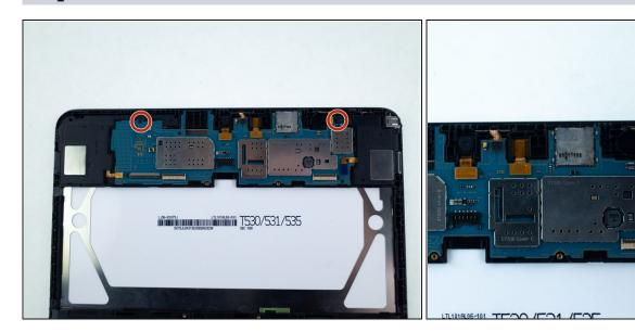
• Remove the two 2.7mm Phillips #00 screws from the motherboard.
