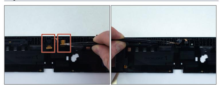
Pull up on the cameras with a pair of tweezers to remove.
