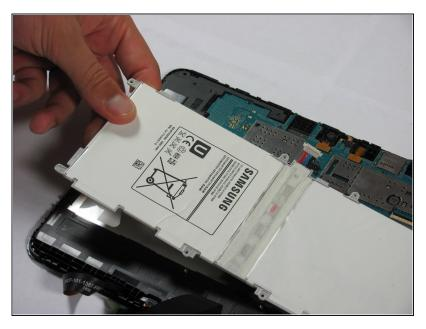
• Once the battery is loose, lift it out of the device.
