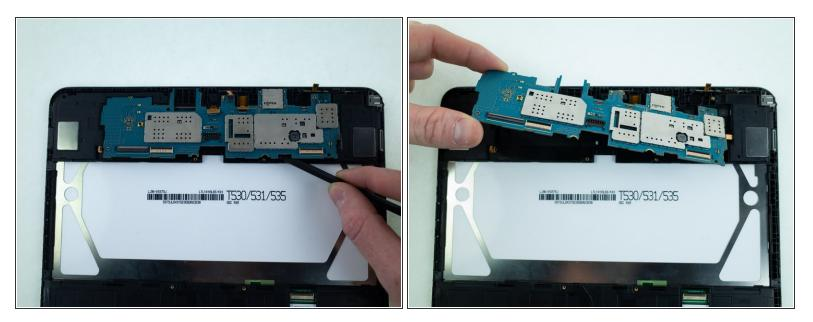
• Use a spudger to pry up the motherboard, and remove it from the device.
