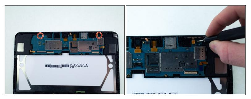
• Remove the two 2.7mm Phillips #00 screws from the motherboard.
