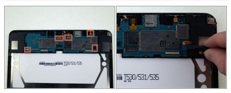
Use the flat end of a spudger to pry up and disconnect the five press-fit connectors from the motherboard.
