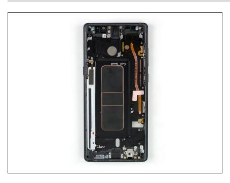
To reassemble your phone transfer all components you removed to the new display assembly with frame.
