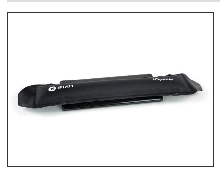
Prepare an iOpener and apply it across the phone to loosen the adhesive beneath the vibration motor at the bottom and the earpiece speaker at the top.
