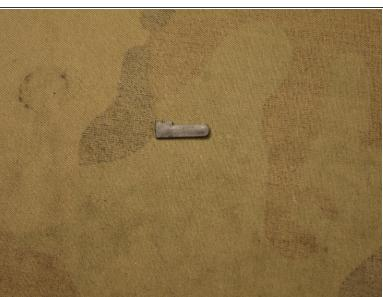
Right underneath the top section that you just removed is the plastic piece that can hold the follower back when you want it to. This piece can simply be grab and poled out to help keep track of everything.
