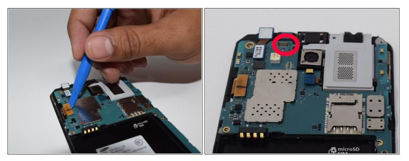
• Use a plastic spudger to disconnect LCD ribbon cable and front facing sensor.
