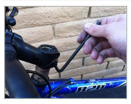
Use a 7/32" Allen Wrench to remove the two bolts; 1 and 2. These clamp the stem to the steerer tube of the fork.
