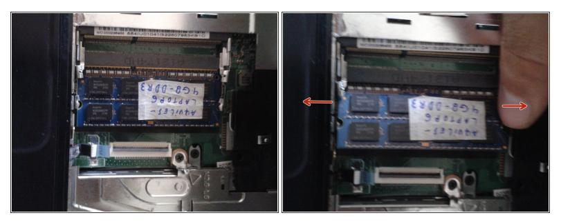
Remove the memory cards by moving the retaining clips in the direction that the arrows are pointing.
