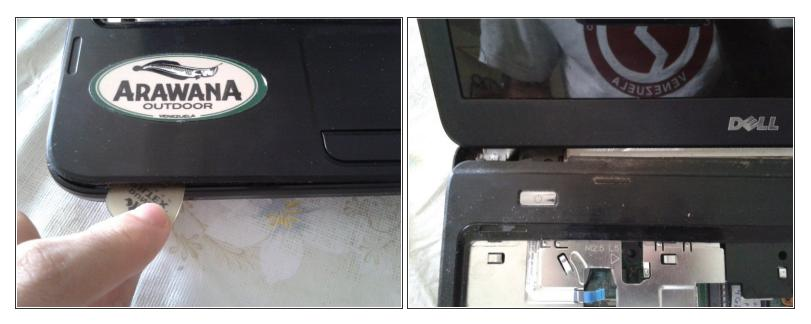
• Use a plastic tool to separate the top of the laptop.
