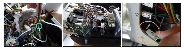
• The Allen screw, which holds the holder of the two thermocouples, was not easy to open...
