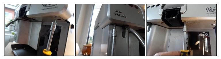
• The screws are situated on the underneath of the cover. This type is held by four screws.
