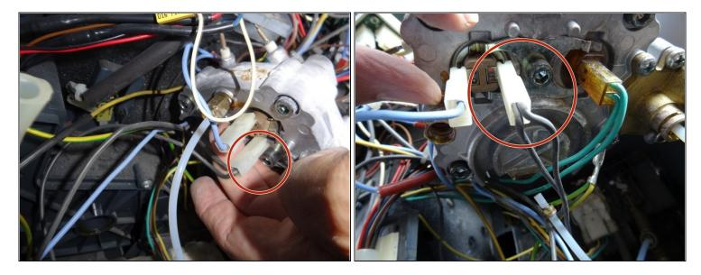
• Disconnect the connector with the two gray cables from the thermal switch.
