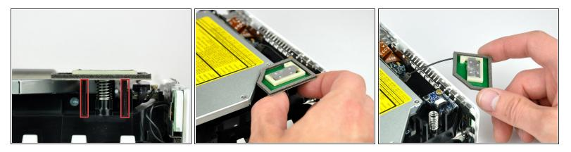
(i) First remove the AirPort antenna (the larger of the two), located near the power button.
