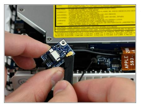
Lift the Bluetooth board off the internal frame and use the flat end of a spudger to pry the Bluetooth antenna cable connector up off the Bluetooth board.
