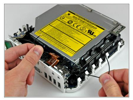
• Pull the Bluetooth antenna cable out from underneath all the cables connected to the interconnect board.
