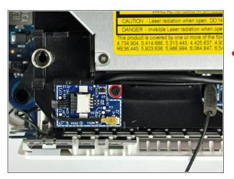
Remove the single Phillips screw securing the Bluetooth board to the internal frame.
