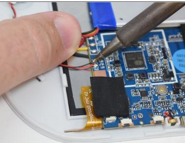
Remove the wires from the motherboard using a soldering iron tool. Here is a link on <u>How To Solder and Desolder Connections</u>.
