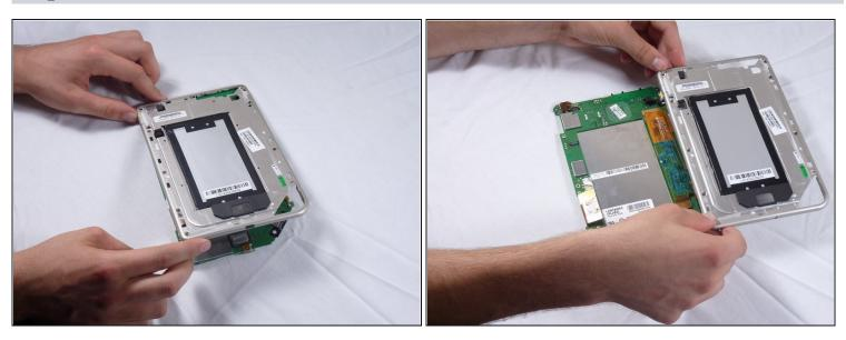
• Carefully lift the silver midframe away from the motherboard and display assembly.
