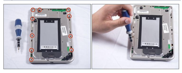
• Using the T5 Torx screwdriver, remove the ten T5 screws from around the edges of the silver midframe.
