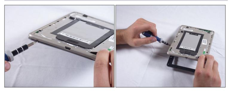
• Using a spudger or plastic opening tool, carefully pry the screen bezel away from the silver midframe.
