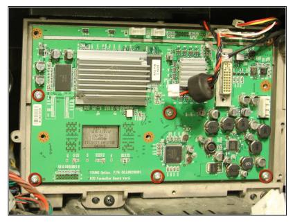
Remove the five remaining 8 mm Phillips #0 screws.
