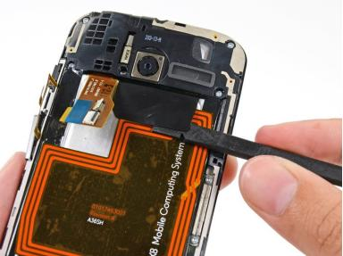
Use the flat end of a spudger to peel the adhesive pull-tab off the top of battery.
