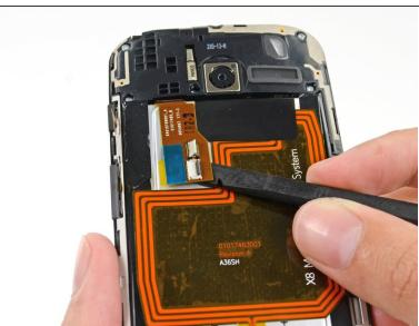
Insert the flat end of a spudger under the interconnect cable to free it from the adhesive holding it to the battery.
