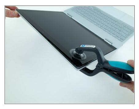
Use an iSclack, or suction cup, to lift up the corner of the display from the case.
